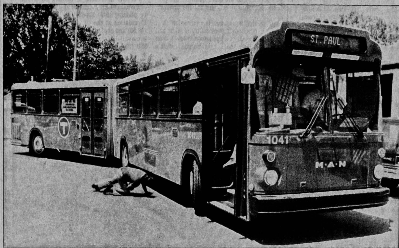
A passenger inspects an oversized Articulated bus, capable of carrying 140 passengers, which Cambus tested Wednesday in hopes that the model would handle more riders when enrollment increases in the fall.
