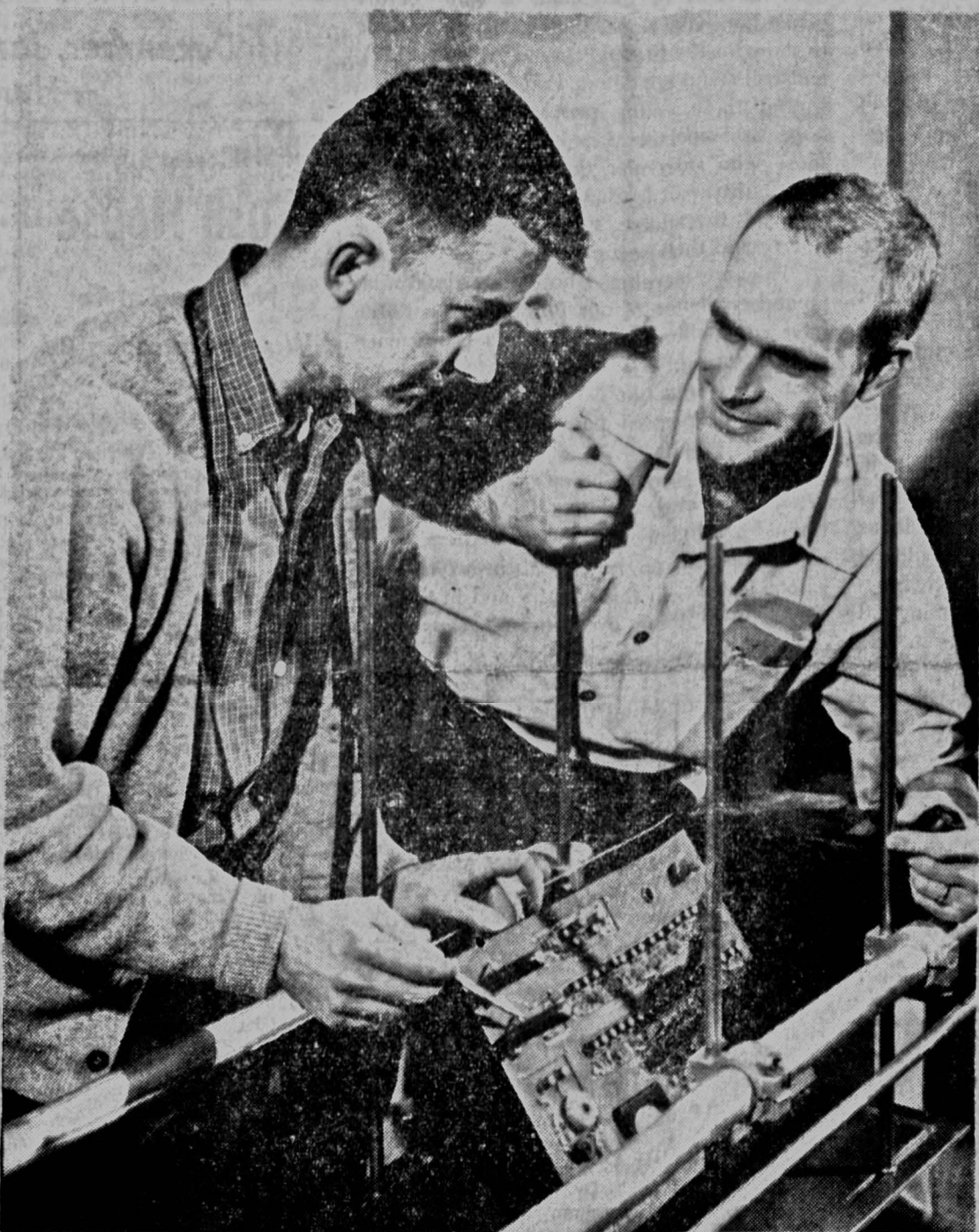
AT RADIATION RIG where the lunar probe payload stood a final test three weeks ago, student assistant Louis Frank, A3, Fort Madison, and Prof. Ernest Ray show a "breadboard" lineup of electronic parts and circuits like those within Pioneer IV.—Daily Iowan Photo by Katie Harris.
