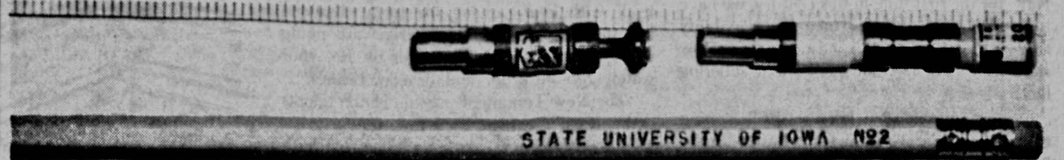
TINY TUBES WITH BIG RESPONSIBILITIES—Size of specially constructed geiger counters aboard Pioneer IV is dramatically indicated by pencil along side. Within the moon-sun probe the
